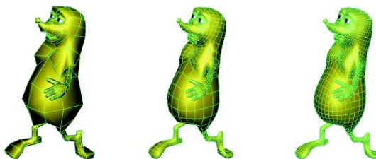
Figure 1: Original mesh and its level 1 and level 2 subdivisions applying the smoothing step once and twice, respectively.
