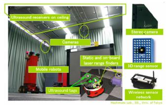
Fig. 1. Intelligent Space with Distributed Sensors and Mobile Robots.
