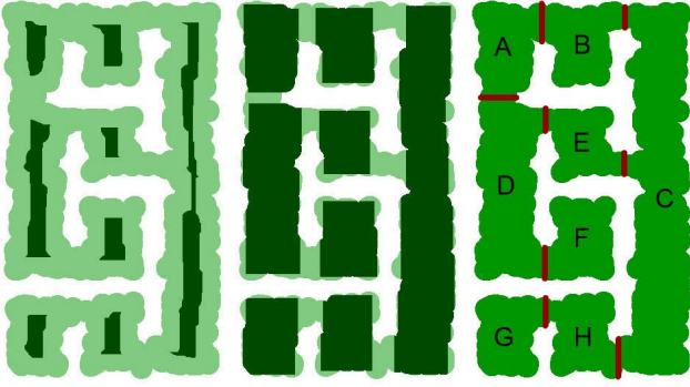
Fig. 9. The eroded (left) and dilated (center) maps. The final decomposed map can be seen on the right.
